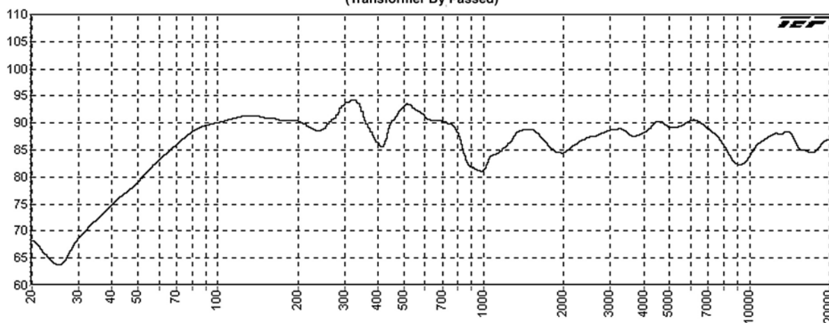
FAP62T Frequency Response (Transformer By Passed)
